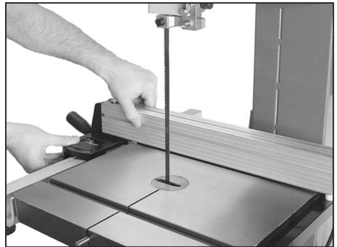
Figure 12. Installing fence onto rails.
